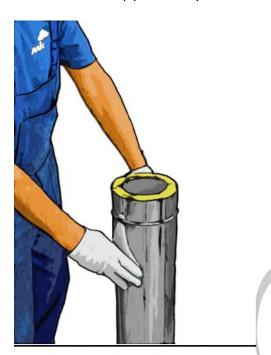
2. Prepare another pipe. Orient the second pipe with its female end pointing down.
